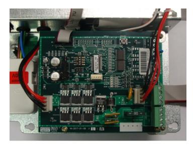
This information is applicable to the AFP2800, IFS2600 panels and the NPS series of standalone/supplies that are fitted with the PSI (Power Supply Interface) board as shown above.
