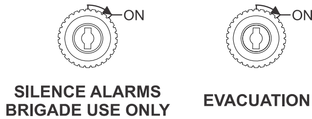
Figure 2.15 Bulgin Switches in their default (OFF) position
